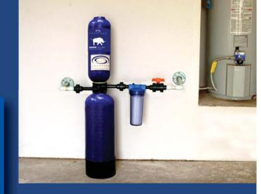
Comes complete with main filter unit, pre-filter, installation kit, shut-off valve and required hardware. The Rhino requires only 45 in. of vertical clearance and has a diameter of 10 in. at the base. Typical installation is 1.5 to 2.5 hours by a licensed plumber and is usually done in your basement, garage, or water heater closet. The main filter unit is easily replaced (no plumber needed) every three years.
